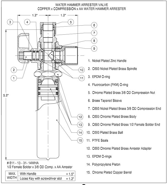
Working Pressure: 250 psi / 250°F depending on pipe material.
